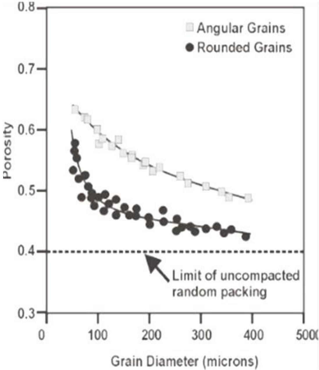
Fig. 3: Porosity and grain size relation
