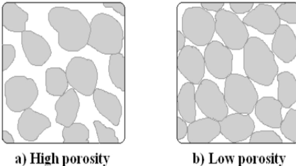
**Fig. 2: The porosity conditions**
