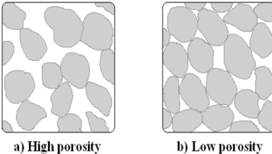
**Fig. 2: The porosity conditions**
